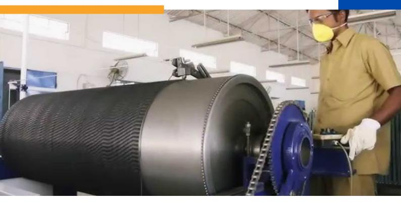
Lakshmi Card Clothing is a well-known Indian company that specializes in manufacturing card clothing products for the textile industry. Card clothing is a crucial component in carding machines, which are used in the textile manufacturing process to separate and align fibers to prepare them for subsequent processes like spinning and weaving.
